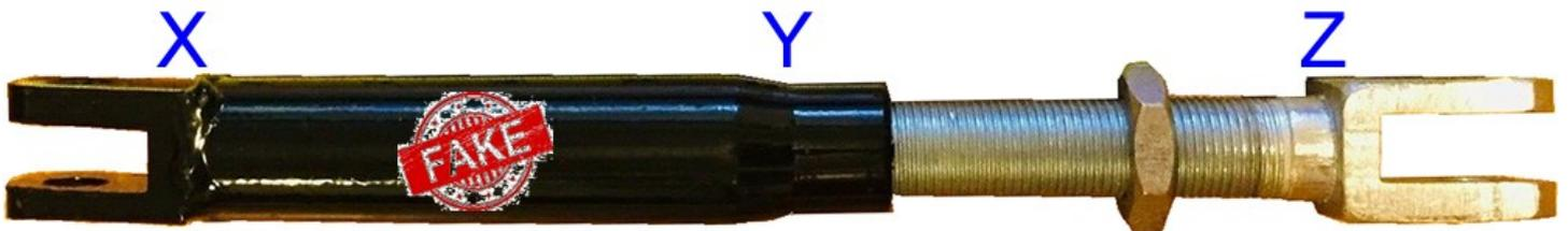
This second example is very worrying indeed. It pretty much demonstrates how not to make this part. The clevis X is again surface welded rather than press fitted, the transition (Y) has stress introduced by the sharp angles during manufacturing. It appears in order to save a little in the production costs the transition parts are made in bulk separately to the main tube and then welded on later. The clevis (Z) has been produced separately to the thread section and then welded on.
